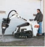
Hydraulic Breaker Break up asphalt, concrete and other hard surfaces; smash through walls. Exceptional power.
