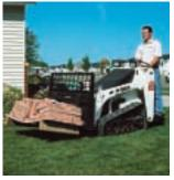
**Pallet Fork** Handles palletized material and long objects, such as lumber and fence posts.
