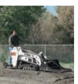
Landplane Grades, levels, transports material, breaks up hard ground, peels sod.
